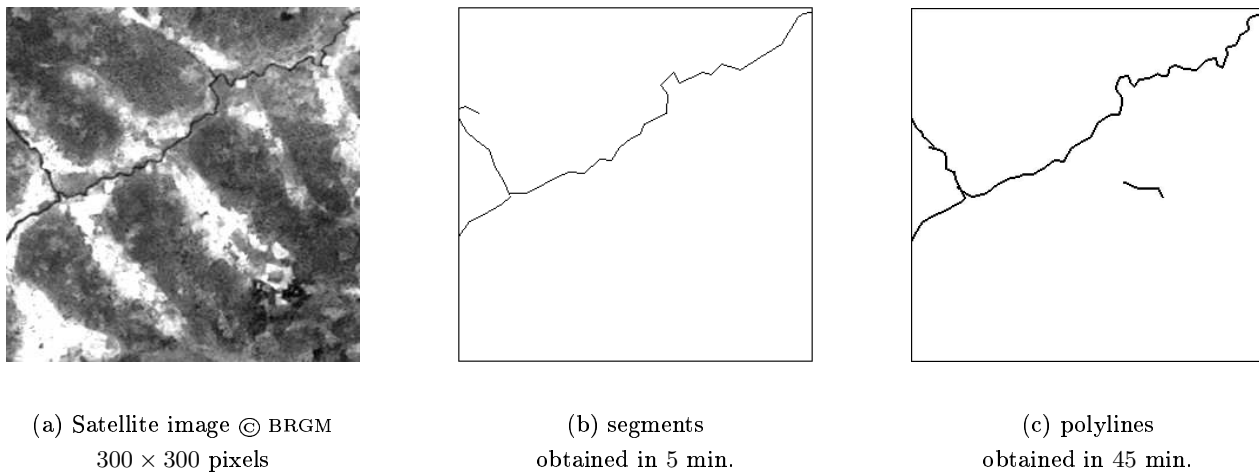
Figure 12: River extraction from a SPOT XS2 image (20 meters of resolution) provided by the French Geological Survey (BRGM): (b) using the segment process “Quality Candy”; (c) using the polyline process “CAROLINE”.
