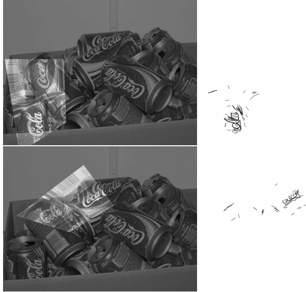
Figure 28: “Coca-Cola” experiment: maximal meaningful groups (last two among five). Their -\log_{10}(NFA) is respectively 3.39 and 4.60. Both of them correspond to a Strobe effect, since the lower part of “oca” is identical to the lower part of “ola”. Left: the registered images. Right: registered pieces of level lines.
