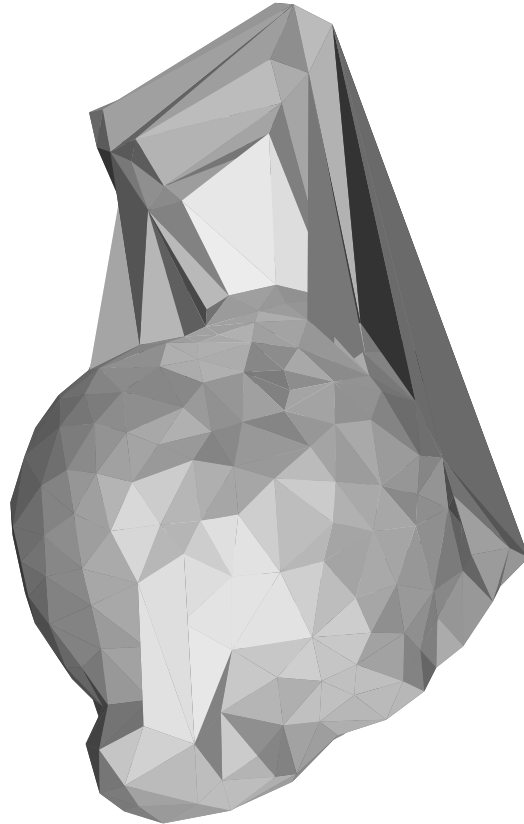
Figure 9: Sculpture result : We have added topological constraints and a priority queue to make our algorithm a sculpture algorithm. The weight of a half-facet can be seen as some measure of the Gabriel property. The original shape could not be extracted. This figures out the topological clamping of a sculpture algorithm.
