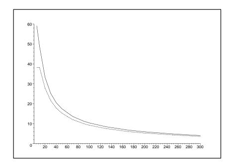
Figure 7: average fraction of nodes belonging to the MPR dominating set (plain), fraction of nodes belonging to the dominating set with rule 2 (dashed), versus density.
