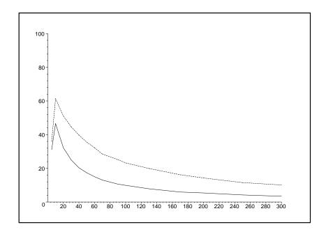
Figure 3: average fraction of nodes in the network implied in an MPR flooding, with greedy algorithm (plain) and with in-id algorithm (dashed), versus density.
