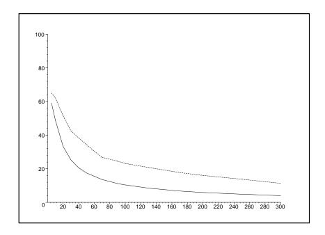
Figure 5: average fraction of nodes which are in the MPR dominating set, with greedy algorithm (plain) and with in-id algorithm (dashed), versus density.
