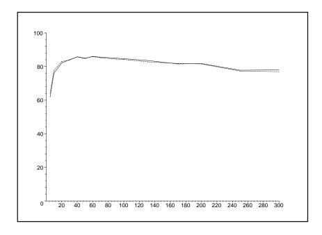
Figure 4: average fraction of nodes which are MPR of at least one node in the network, with greedy algorithm (plain) and with in-id algorithm (dashed), versus density.
