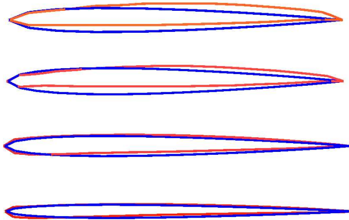
Figure 15: Isolated wings of the Supersonic Business Jet. Optimization Strategy I. Shape optimization shown at the four wing sections. From top to bottom: Sections A, B, C and D. In blue, the original shape.
