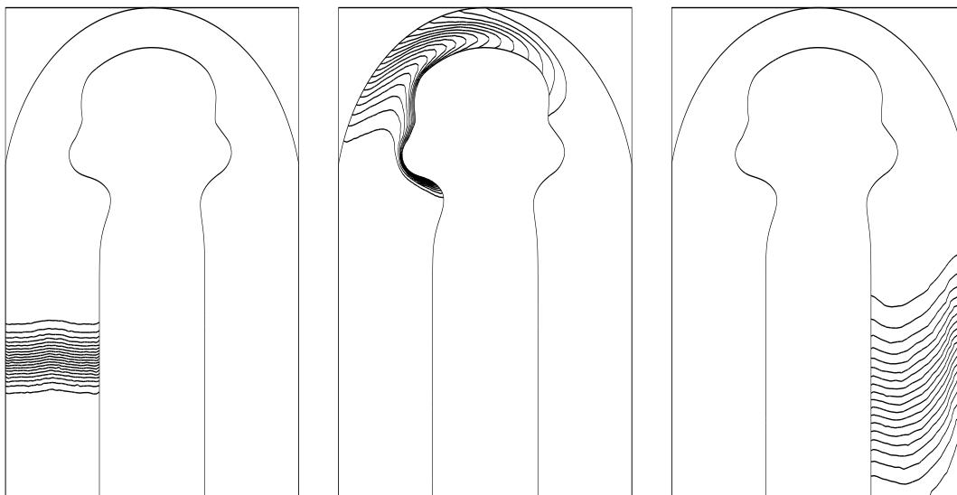
Figure 9: Second class of optimized shapes for the 180 degree turn. Here again, larger curvature variation introduces more dispersion in the advection band away from walls.
