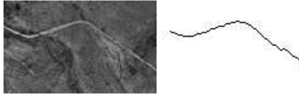
Figure 3: right, the road joining two extremities given by ELIESER ; left, the corresponding piece of SPOT image.
