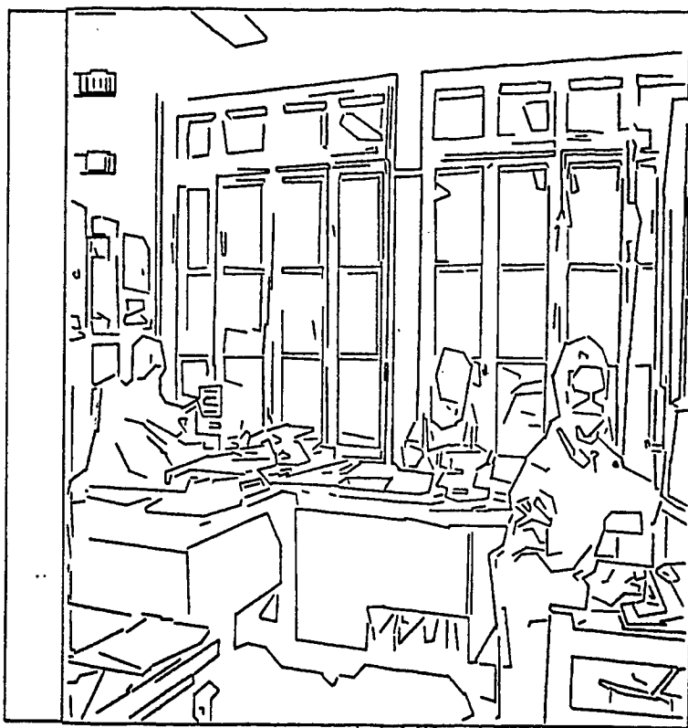
Figure 12: Polygonal approximation of the edge points of a stereo pair of an office room observed in position 1
