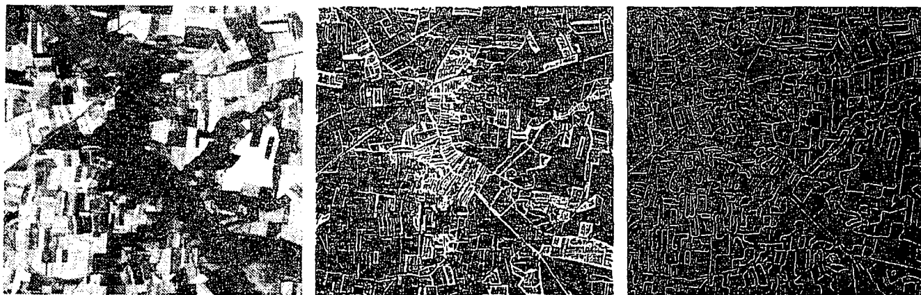
Figure 6: spot image, points with g(\alpha) lower than 1.8, Canny's edges
