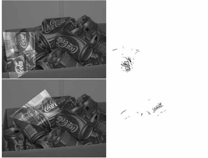
Figure 28: “Coca-Cola” experiment: maximal meaningful groups (last two among five). Their -\log_{10}(NFA) is respectively 3.39 and 4.60. Both of them correspond to a Strobe effect, since the lower part of “oca” is identical to the lower part of “ola”. Left: the registered images. Right: registered pieces of level lines.
