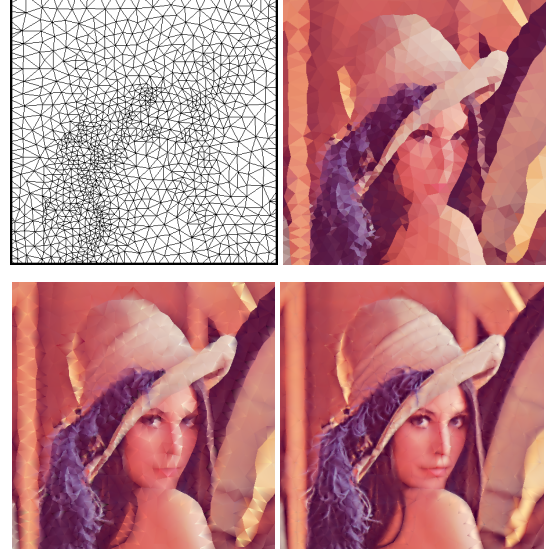
Figure 6: Trixels with the attached pre-integrated higher-order representation of degree 0, 1 and 2 (2000 trixels).
