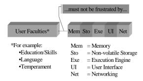
Figure 3. The resource layer serves as the foundation for the application software. It contains the available computational resources and assumed user skills and abilities that developers can count on being present.
