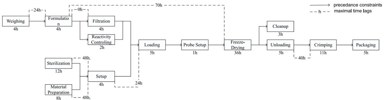
Figure 4: freeze-drying process
