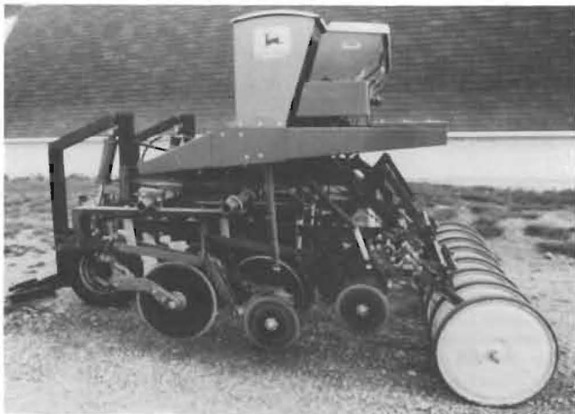
Figure 1. No-till experimental drill designed and constructed to evaluate different types of furrow openers and packer wheels in no-till research.
