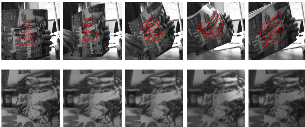
Figure 11: Visual tracking of a deformable surface in a sequence of 400 images acquired with an uncalibrated camera. The top row shows the (6 \times 5) regular grid used to track the tracked area of interest in the image sequence. The bottom row shows the area of interest registered with respect to the template.
