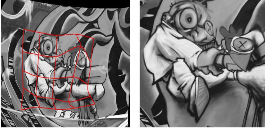
Figure 2: Visual tracking with the Gauss-Newton minimization. The image on the left shows the transformation of the regular grid after 40 images of the sequence. The registration fails due to the real-time constraints. This is clearly visible in the right image where the warped area of interest in the reference frame is not equal to the reference template.
