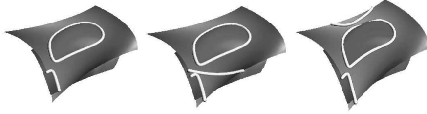
Fig. 6. First example. Left and center: Result of the resultant method after and before eliminating phantom branches. Right: result of the approach using approximate implicitization.
