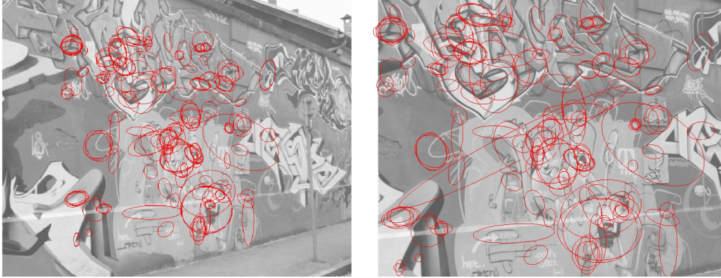
Figure 6: A comparison with Harris-Affine interest point detector, with GLOH descriptor [11] (K. Mikolajczyk's implementation.) The same robust matching algorithm as in Fig. 4 and 5 is used: threshold of step 1) is set so that (almost) no false detection can be seen, leading to 196 inliers to the estimated homography. 4093 descriptors were extracted from the left image, and 4376 from the right one. Although the algorithm is affine-invariant, this gives almost the same proportion of retrievals as in Fig. 5.
