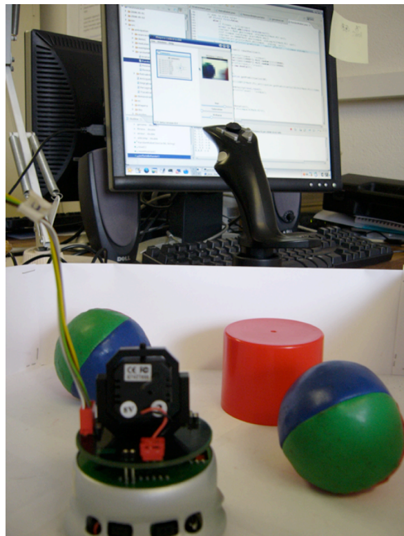
Fig. 11. Learning by demonstration experimental setting. Foreground: Khepera robot, red target, two obstacles. Background: joystick and control screen.
