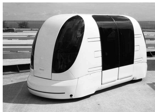
Fig. 1. ULTRA PRT vehicle [1].
