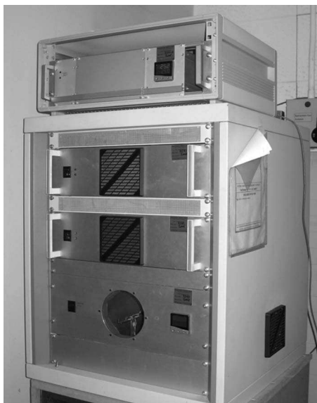
Fig. 10. Environmentally controlled test chamber.
