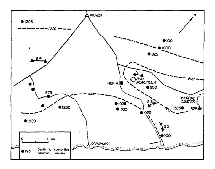
Figure 3. Contoured values of second-layer thickness, or depth below sea level to conductive basement, in meters.
