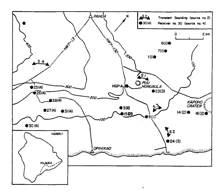
Figure 1. Map of the lower East Rift zone of Kilauea volcano, Hawaii, showing prominent roads and topographic features. Also shown are the locations of the grounded-wire sources and horizontal-loop receivers used in the soundings interpreted in this report.
