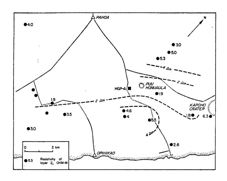
Figure 2. Contoured values of second-layer resistivity, in ohm-m.
