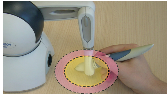
Figure 5: Simulating the RubberEdge hybrid technique with the Phantom haptic device. A 2D simulated haptic surface constrains the pen movement and the elastic zone is created using force feedback.
