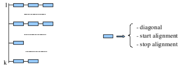
Figure 5: Linked lists of three ungapped alignment fields.
