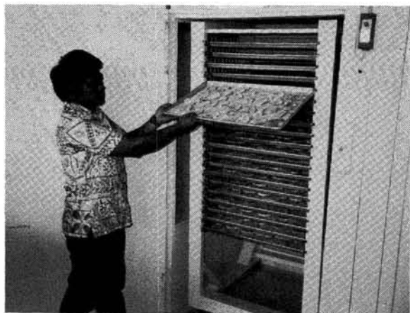
Roy Nakanishi examines pineapple slices drying in an oven powered by waste geothermal heat.
