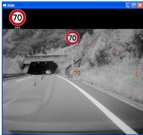
Fig. 2. Example of E.U. speed-limit sign detection and recognition with our initial system. All detected circles are shown (in red or green), and the candidate digits segmented inside them are outlined in red. The speed signs recognized on the current image are shown on the top black zone, with their associated confidence, and the currently validated speed limit is superimposed on top-center of image.
