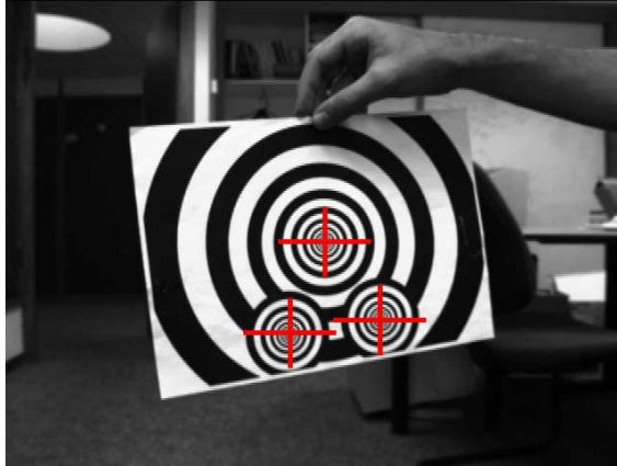
(a) Circular 3-pattern SSL target showing results of landmark identification.
