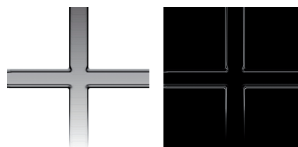
Figure 3: “Simple” image texture: original image and discontinuity map by Sobel filtering.
