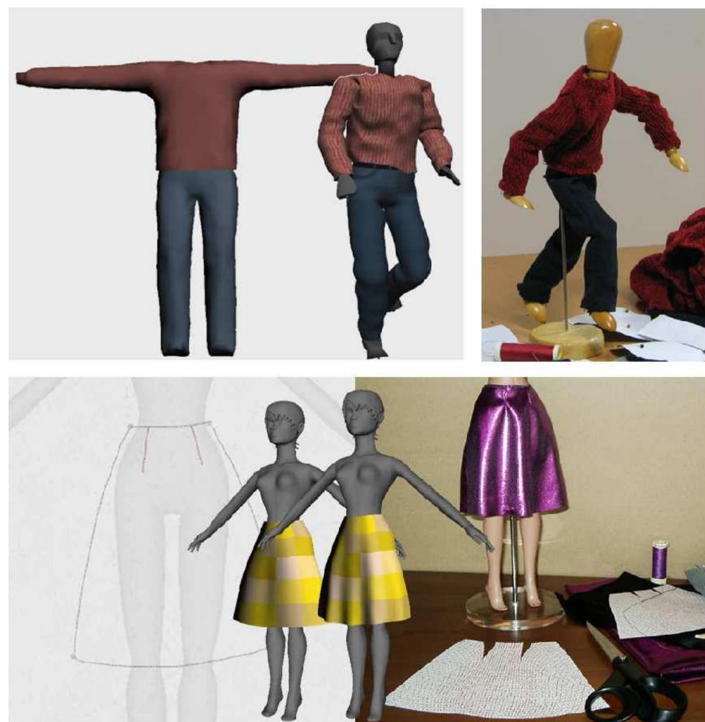
Figure 12: Comparison between the virtual clothing we designed and real replicas sewn from the patterns we output.
