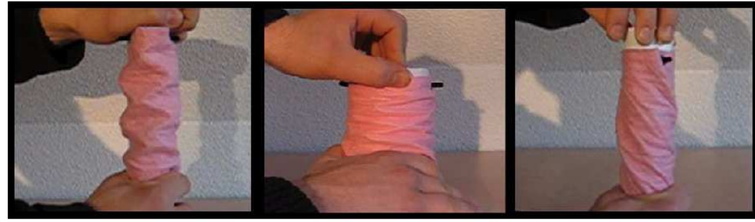
Figure 6: Buckling phenomena for a cylinder of fabric. Diamond shape patterns (left and middle) appear under axial compression. Twist patterns (right) made of parallel oblique wrinkles appear when one end of the panel is twisted.
