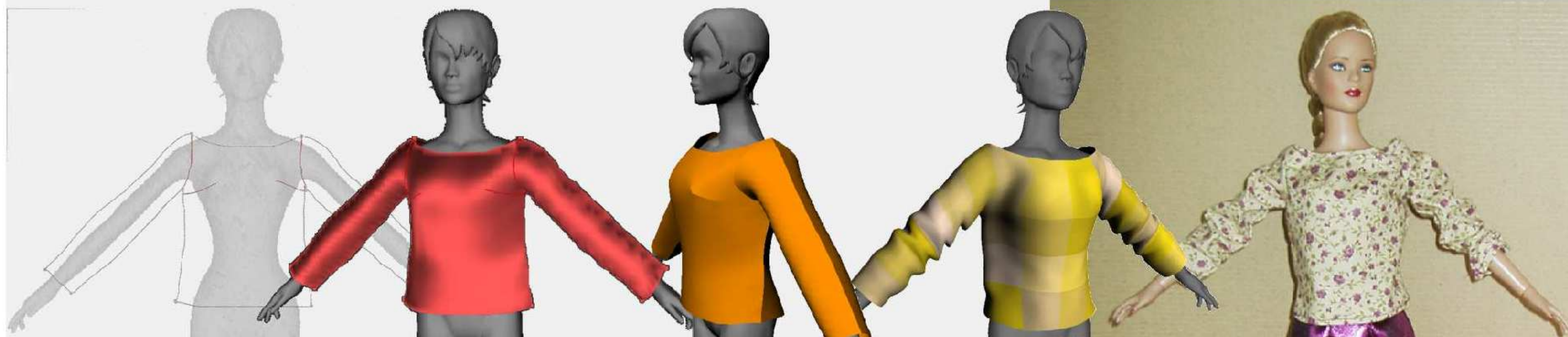
Figure 1: From sketch to garment. Left to right: sketched contours and darts; 3D shape computed using distance field; piecewise developable surface; final virtual garment, compared with the real one sewn from the 2D patterns we output.
