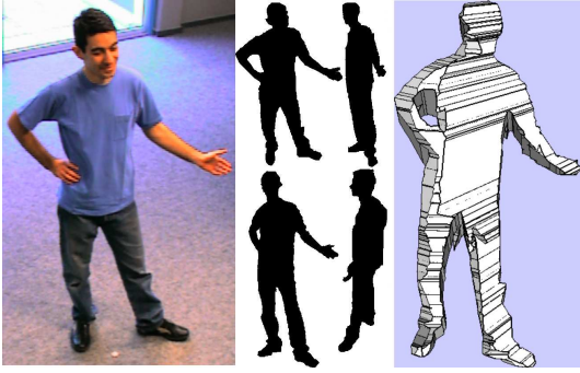
Figure 6: Real time reconstruction of a real person with 4 cameras and the exact connectivity approach.
