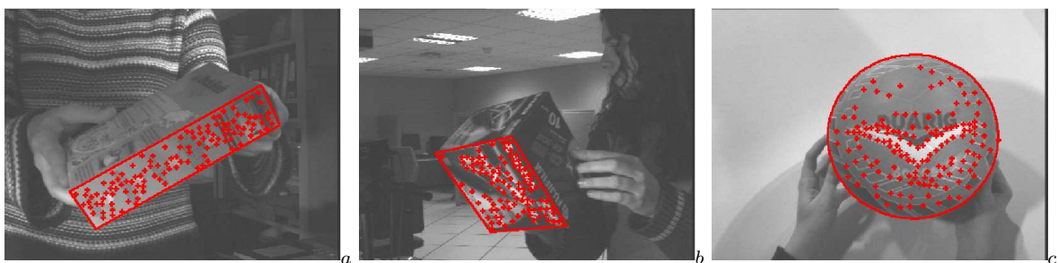
Figure 4: Texture model for a face of: (a) a rice box, (b) a DVD box, (c) a ball
