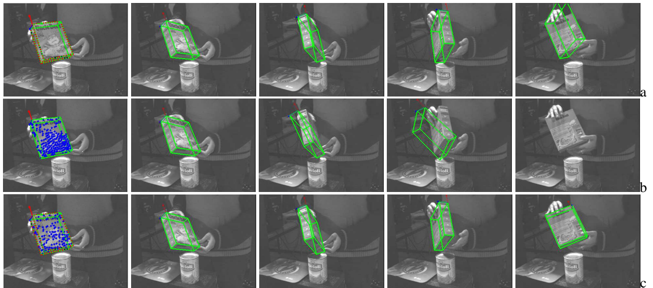
Figure 18: Rice box sequence. Images for (a): the edge-based tracker, (b): the texture-based one, (c): the hybrid one. Only the hybrid tracker succeeds to track correctly the object all along the sequence, despite the specularities and the misleading environment. The grey level samples are represented in the first image by blue crosses and the edge location by red points.
