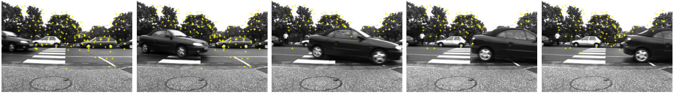
Fig. 6. Every second frame of a sequence from experiment 1 demonstrates robust feature (yellow crosses) tracking resumption after occlusion by a passing car.
