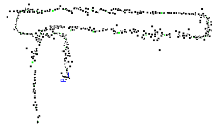
Fig. 12. Larger noise in the reconstructed robot poses where all features are far away in experiment 3.
