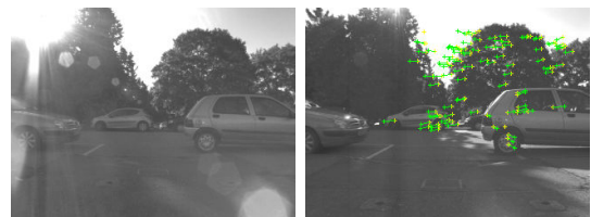
Fig. 13. Sun shining into the camera in the reference image (left), but not in the current image (right) during navigation in exp. 3.
