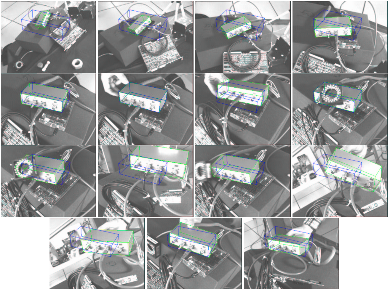
Figure 6: 2D 1/2 visual servoing experiments: on these snapshots the tracked object appears in green and its desired position in the image in blue. The six first images have been acquired during an initial visual servoing step where the object is motionless. In the reminder images, object is moving along with the robot.
