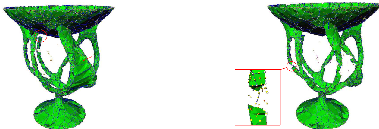
Figure 5: Assessing the importance of persistence (a) At t_r = 1.7, t_p = 0 , a fin between two handles of the vase model is observed, while one back handle is disconnected—circled region. (b) At t_r = 2, t_p = 1.02 , the fin is gone. Note also the preservation of the homotopy type of a solid handle, which is reconstructed as a polyline.
