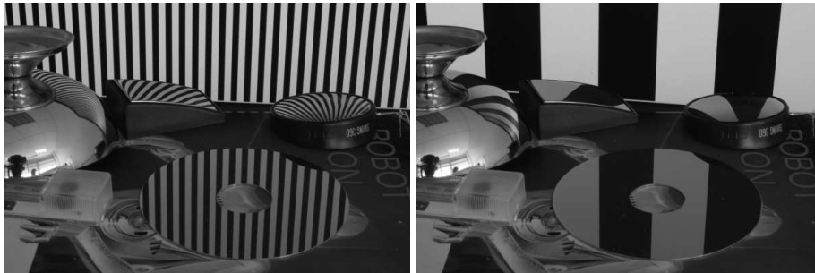
Fig. 3. Two of the images used for the reconstruction of the planar hard drive platter.
