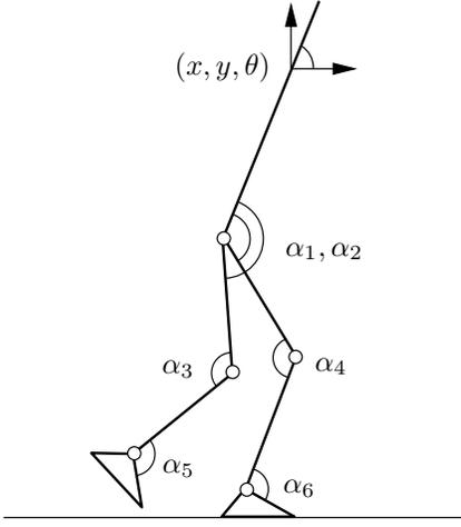
Figure 1: The configuration of a 6-DOF planar biped robot can be expressed through 9 variables, 3 for the global position of the robot  $(x, y, \theta)$  and 6 for its internal shape  $(\alpha_1, \dots, \alpha_6)$ , to obtain the state vector  $q = (x, y, \theta, \alpha_1, \dots, \alpha_6)^T$ .
