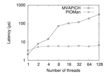
Fig. 4. Multi-threaded latency test on BORDERLINE
