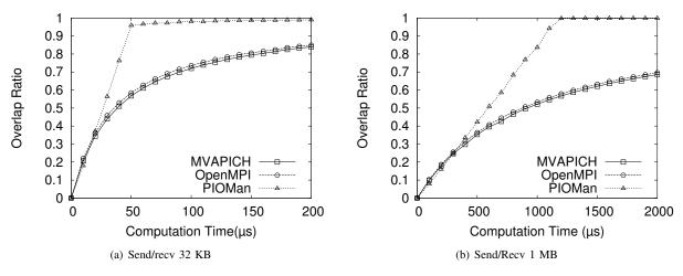
Fig. 7. Overlap Performance (computation on both sides)
