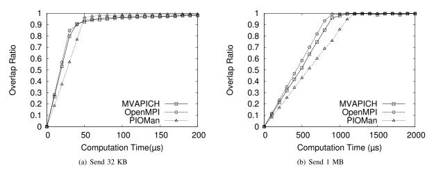
Fig. 5. Overlap Performance (computation on sender side)
