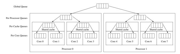
Fig. 2. Hierarchical lists mapped to a machine topology
