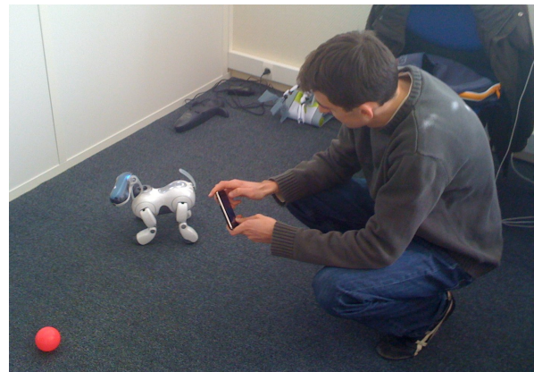
Figure 6: In our new prototype, the iPhone accelerometer can be used as a TUI to orient the robot head.
