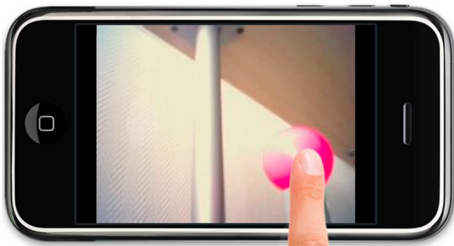
Fig. 2. The iPhone gestures interface with "interactive" video stream, where users can define "trajectories" (through strokes such as swipe or tap) interpreted as commands. The screen of the device equally allows to provide visual feedback such as arrow showing the movements of the robot.
