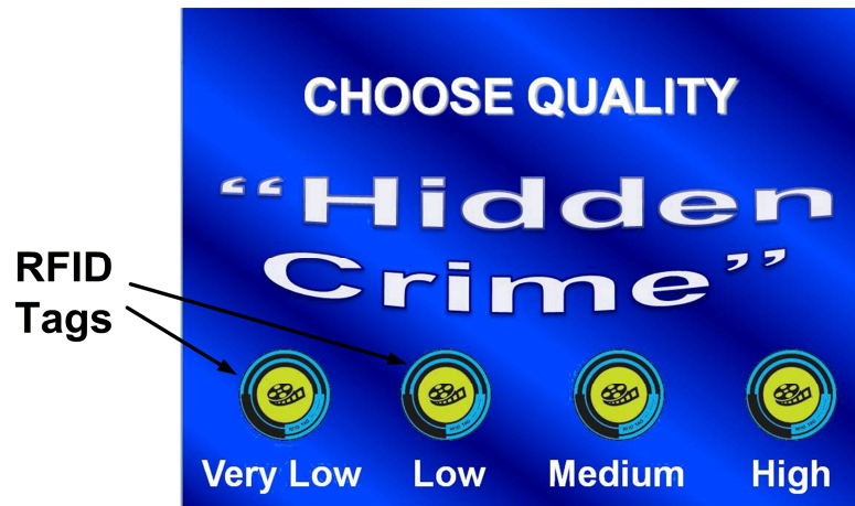
Fig. 2. Physical user interface for providing user preferences used by Davidyuk et al (2008a).
