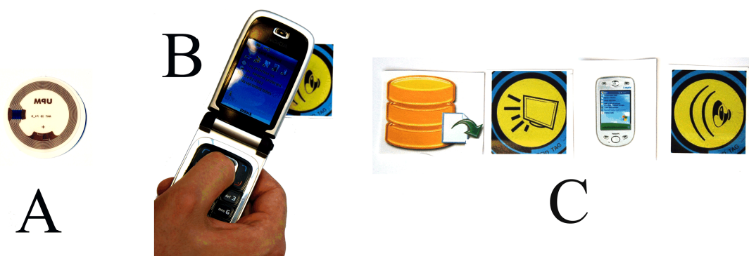
Fig. 4. Sticker with RFID tag (A), RFID reader (B), and set of service cards (C).
