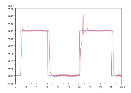
Figure 2: Forward speed of the CoM (red) and reference speed (blue) for the motion of Fig. 1.
