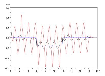
Figure 9: Lateral speed of the CoM (red), mean value of this speed over prediction horizons (grey) and reference speed (blue) obtained with the Predictive Control scheme (31).
