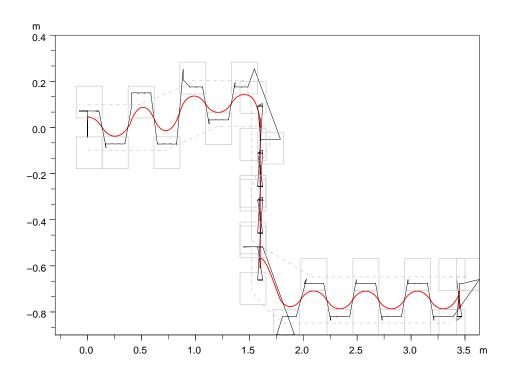
Figure 1: Foot step placement and ankle motion (grey), Center of Pressure (black) and Center of Mass (red) positions for the sample motion described in Section 6, obtained with the Predictive Control scheme (17).
