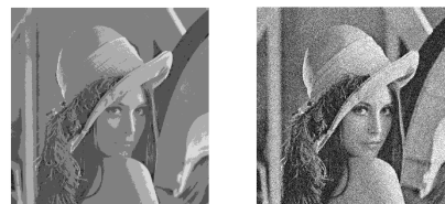
Reconstruction quality with a non-dithered (left) and a dithered (right) bioinspired quantizer.
