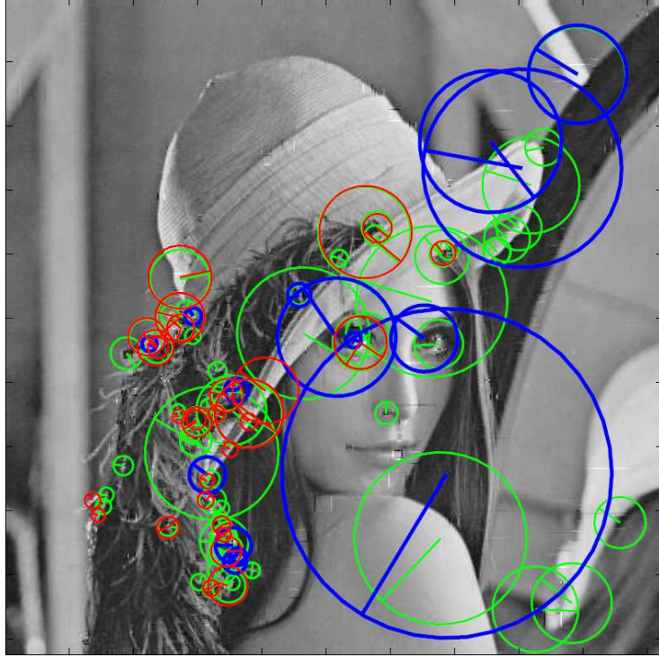
Figure 4: Representation of a subset of keypoints: the center is the keypoint location, the radius is proportional to the scale, and the dominant orientation is given by the represented radius. In blue: unchanged keypoints; in green: keypoints removed by KPR-attack; in red: created keypoints.
