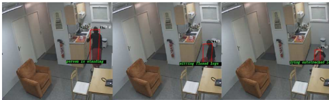
Figure 13. Recognition of the "falling down" event
