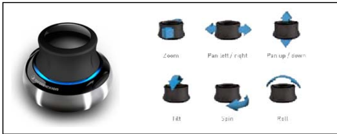
Figure 3: The SpaceNavigator and its six dofs.
