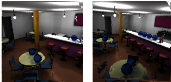
Fig. 8. Two frames from a Render Cache interactive session running at 2 Hz, using the output of our system. We are turning left; some artifacts remain where samples are not yet available.
