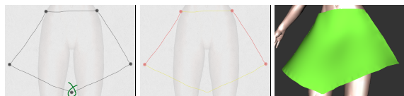
Figure 2: (left) The user has drawn a few lines to indicate the shape of the skirt; the corner-detector has detected a breakpoint that the user does not want. The user will make a deletion gesture (a curve in the shape of an \alpha enclosing the mistaken point) to delete it. (middle) The user has deleted the breakpoint, and the lines have been classified: the silhouettes are in red and the borders in yellow. (right) The surface inferred by the system once the user has required a reconstruction.
