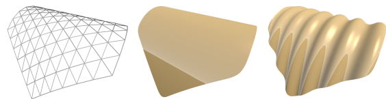
Figure 8: A regular mesh (left) subdivided by LS^3 using default normal computation (middle), and after tweaking the normals (right).
