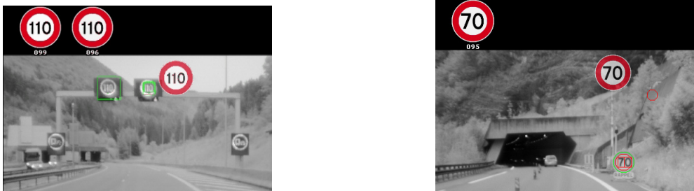
Figure 1. By nature, variable speed limits and roadwork temporary speed limits cannot be obtained from the static cartographic information.
