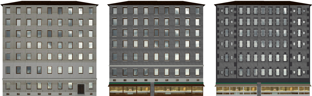
Figure 10: This figure shows the principle of iterative refinement in design. The left building does not have any specific attributes, the middle building has the attribute “shop” and “color variation” applied, and the rightmost building has—in addition to the ones for the middle building—attributes for vertical emphasis on the first and last column and horizontal emphasis on the second and third floor.
