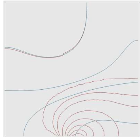
Figure 17: Isolines of the temperature field for a large displacement ( t = 30s ). Blue lines correspond to the simulation, red lines to the fast estimate.
