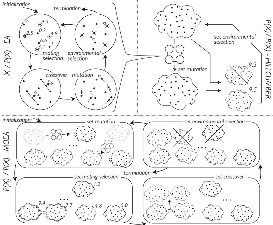
**Fig. 1.** Illustration of different types of MOEAs: (top left) usual view of a MOEA where the operators work on solutions; (top right) a set-based view of the same algorithm; (bottom) an evolutionary algorithm working on sets, i.e., a  $\mathcal{P}(X)/\mathcal{P}(X)$ -optimizer.
