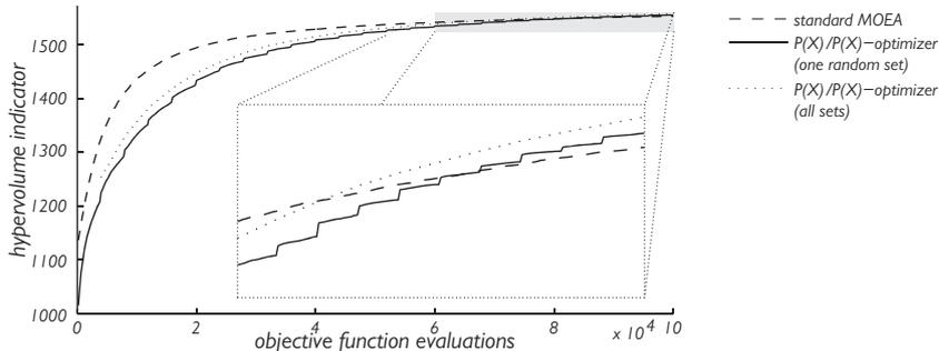
**Fig. 4.** Hypervolume indicator values of the  $\mathcal{P}(X)/\mathcal{P}(X)$ -optimizer variant A1 in comparison to the standard MOEA averaged over 30 runs over time. For the A1 variant, both the overall hypervolume of all solutions and the indicator value of one randomly picked set are shown. The insert shows a detailed view of the last time period.
